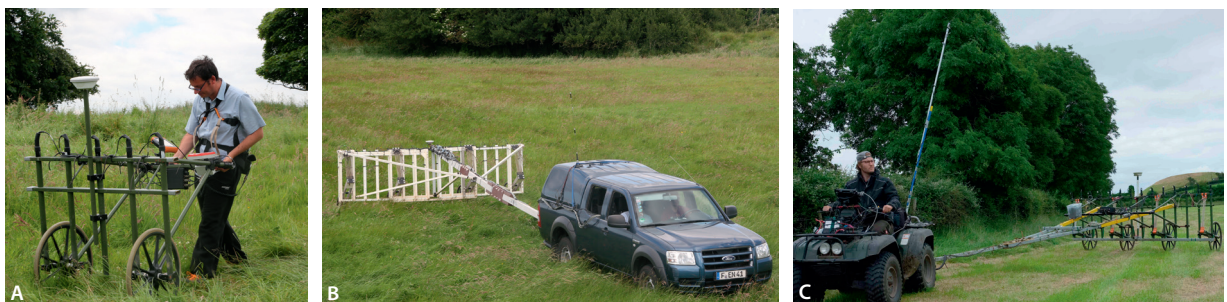
Fig.5. A The 5-channel magnetometer (SENSYS MAGNETO®-MX ARCH) at Dowth in 2014. B The SUV-towed 16-channel magnetometer (SENSYS MAGNETO®-MX ARCH) close the enclosure in Dowth. C The quad-towed 14-channel magnetometer (SENSYS MAGNETO®-MX ARCH) at Newgrange 2017. All systems are working with sensors spaced in a 25 cm distance (Photos: Knut Rassmann).
